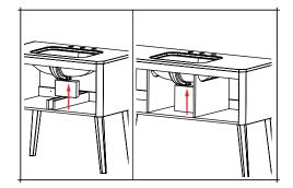
Make all plumbing connections **and check for leaks. We recommend a WA005 low profile waste.** Return the drawers to their respective guides. To adjust the front panel remove the cover cap on the inside drawer.
