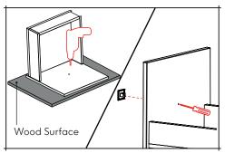
Offer the basin to the countertop and measure the height between the base of the carcass and the bottom of the basin. Prepare a timber block to hold the basin in place.
